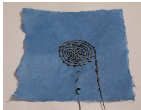
(a) Embroidered speaker made from conductive thread, front.
